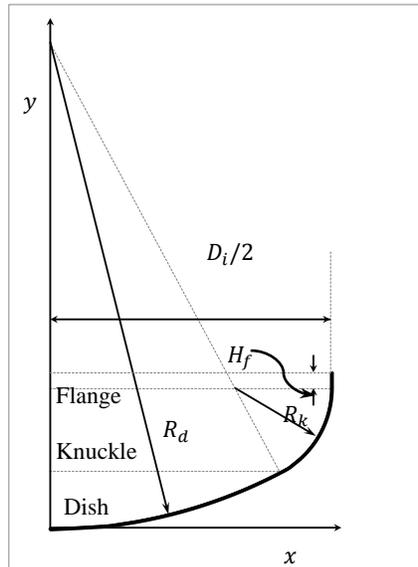
Figure 1. Cross-sectional view of a torispherical head showing the radii of curvature and the coordinate system used for vertically oriented vessels
