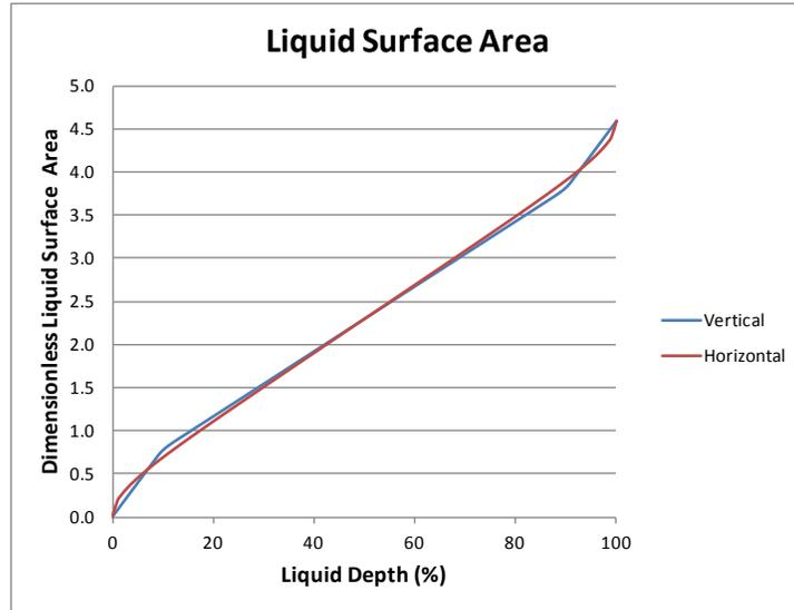
Figure 14. Liquid surface area versus liquid depth for the same vessel oriented vertically and horizontally
