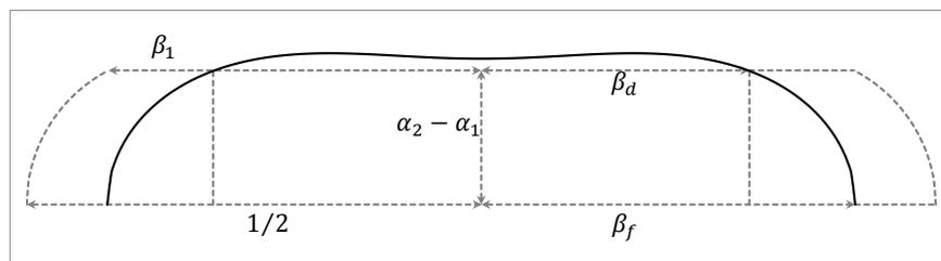
Figure 6. Top view of the knuckle of the left head of a horizontally oriented vessel, rotated 90 degrees clockwise, showing the intersection of the horizontal plane at vertical position  $\delta = (1/2 - \beta_1 + 2f_k)/2$  with the knuckle
