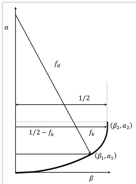
Figure 2. Cross-sectional view of a torispherical head showing dimensionless parameters
