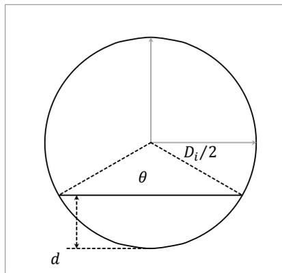
Figure 4. End view of the intersection of a horizontal plane with the cylindrical part of a horizontally oriented vessel
