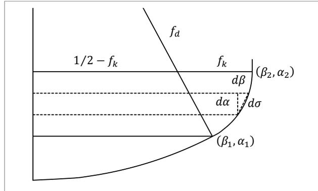
Figure 3. Thin horizontal slice of the knuckle for surface area integral
