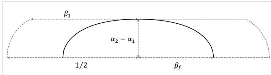
Figure 5. Top view of the knuckle of the left head of a horizontally oriented vessel, rotated 90 degrees clockwise, showing the intersection of the horizontal plane at vertical position  $\delta = 1/2 - \beta_1$  with the knuckle
