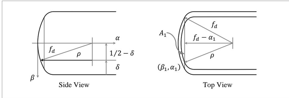
Figure 7. Side view and top view of the left end of a horizontally oriented vessel showing liquid depth
