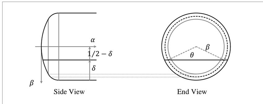
Figure 8. Side view and end view of the left end of a horizontally oriented vessel showing liquid depth  $\delta$
