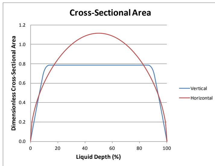
Figure 15. Cross-sectional area versus liquid depth for the same vessel oriented vertically and horizontally
